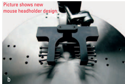
Fig. 12a: Modelling clay for fixing the head of a mouse; b: mouse head holder from Luigs & Neumann
