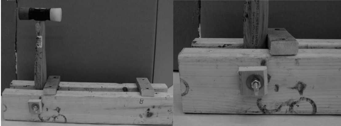
Figure 2. Construction of impact spatter device.
