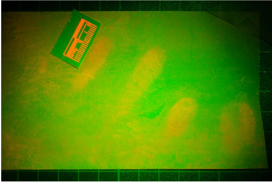
Figure 25: Thermal side sample after processing with fluorescent magnetic powder
