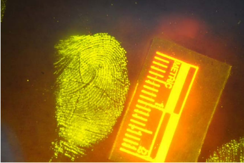
Figure 8: A close-up photograph of a 2-week-old non-thermal side latent print developed with PDMAC® paper in sequence 5
