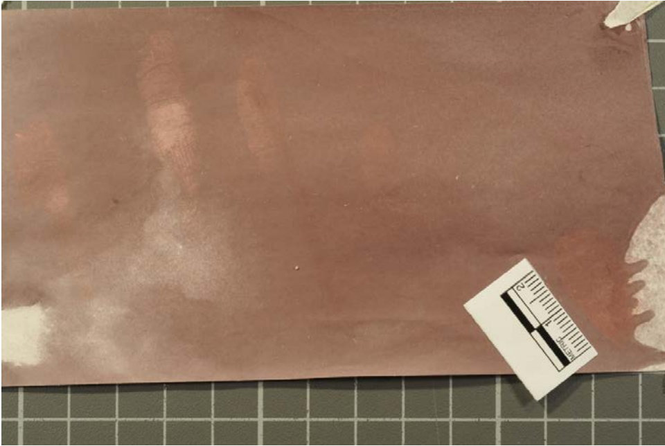
Figure 2: An overall photograph of 24-hour fingerprints that were processed with the oven, 1,2-indanedione/zinc chloride and lastly ThermaNin®
