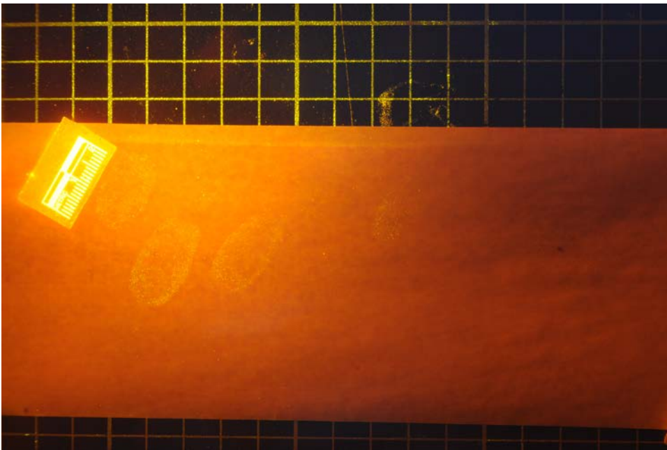
Figure 11: 1,2-indanedione/ zinc chloride development of 3-week old non-thermal side fingerprints
