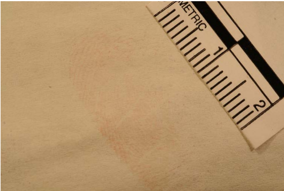
Figure 3: Latent fingerprint developed with ThermaNin® on 2-week-old non-thermal sample
