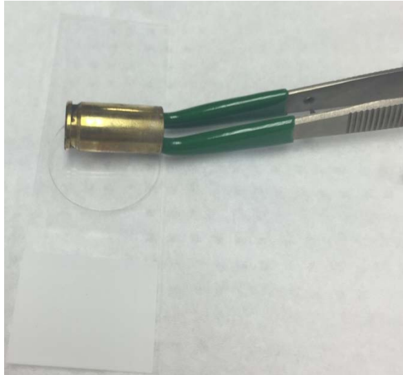
Figure 2 Processing a casing using the tape lift method. Each casing was rolled across a double-sided tape dot with rubber tipped forceps.
