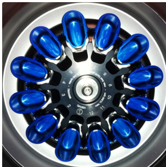
Figure 2: The QIAcube® centrifuge with 12 rotor positions
