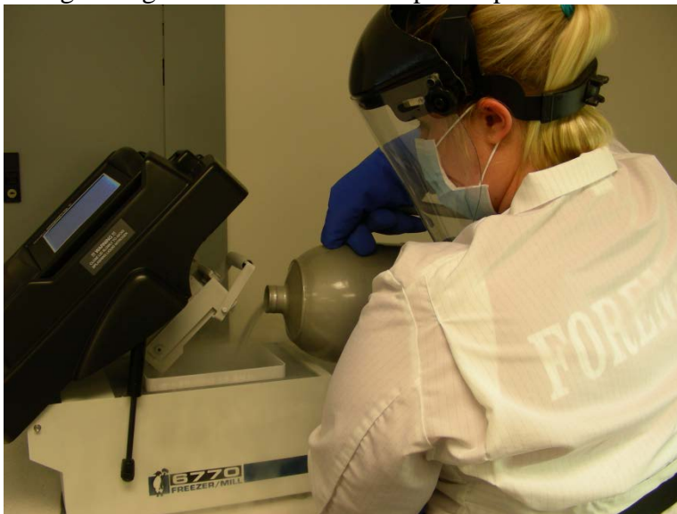
Figure 2: Pouring Nitrogen Into the SPEX Sample Prep LLC® 6770 Freezer Mill
