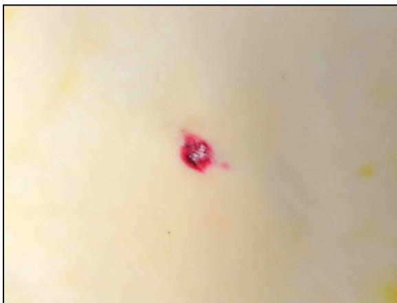
Figure 14 Remington® 110 JHP fired from 8" barrel at 48" distance, Sodium Rhodizonate Test
