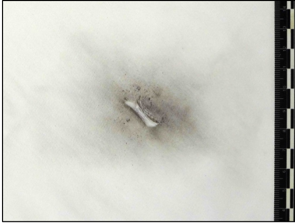
Figure 1 Hodgdon Clays® 3.5 Gr. fired from 2" barrel at 3" distance
