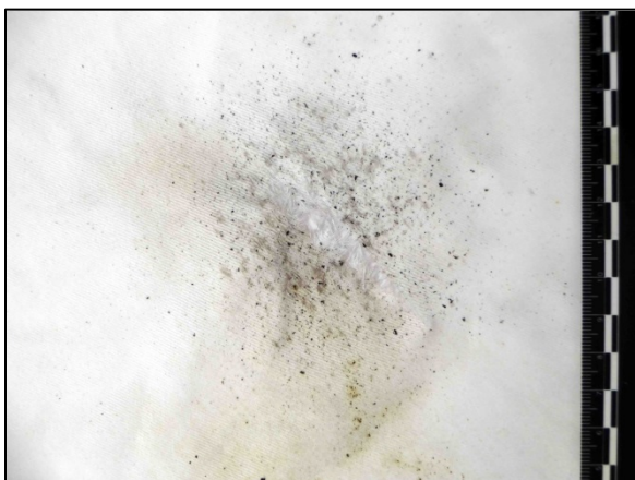
Figure 5 Alliant Blue Dot® 12.0 Gr fired from 2.5" Barrel at 3" distance
