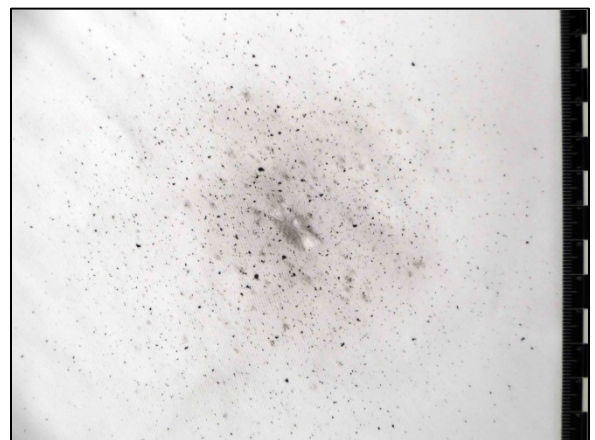
Figure 6 Alliant Blue Dot® 12.0 Gr fired from 2.5" barrel at 6" distance
