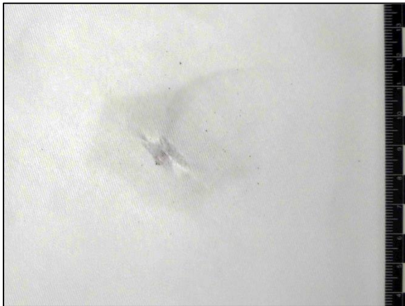
Figure 3 Hodgdon Clays® 3.5 Gr fired from 2" barrel at 9" distance
