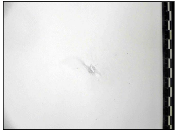
Figure 4 Hodgdon Clays® 3.5 Gr fired from 2" barrel at 12" distance
