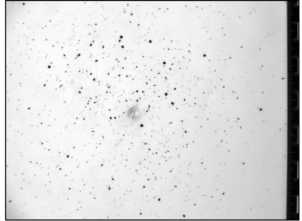
Figure 8 Alliant Blue Dot® 12.0 Gr. fired from 2.5" barrel at 12" distance
