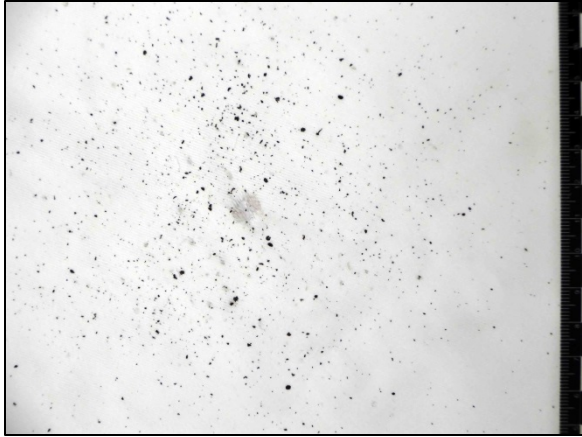
Figure 7 Alliant Blue Dot® 12.0 Gr fired from 2.5" barrel at 9" distance
