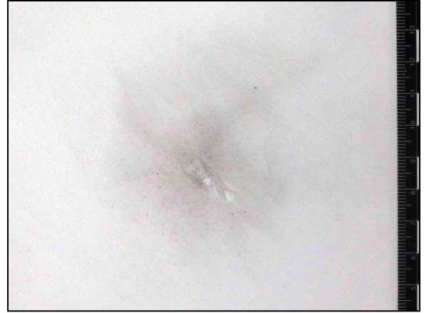
Figure 2 Hodgdon Clays® 3.5 Gr. fired from 2" barrel at 6" distance
