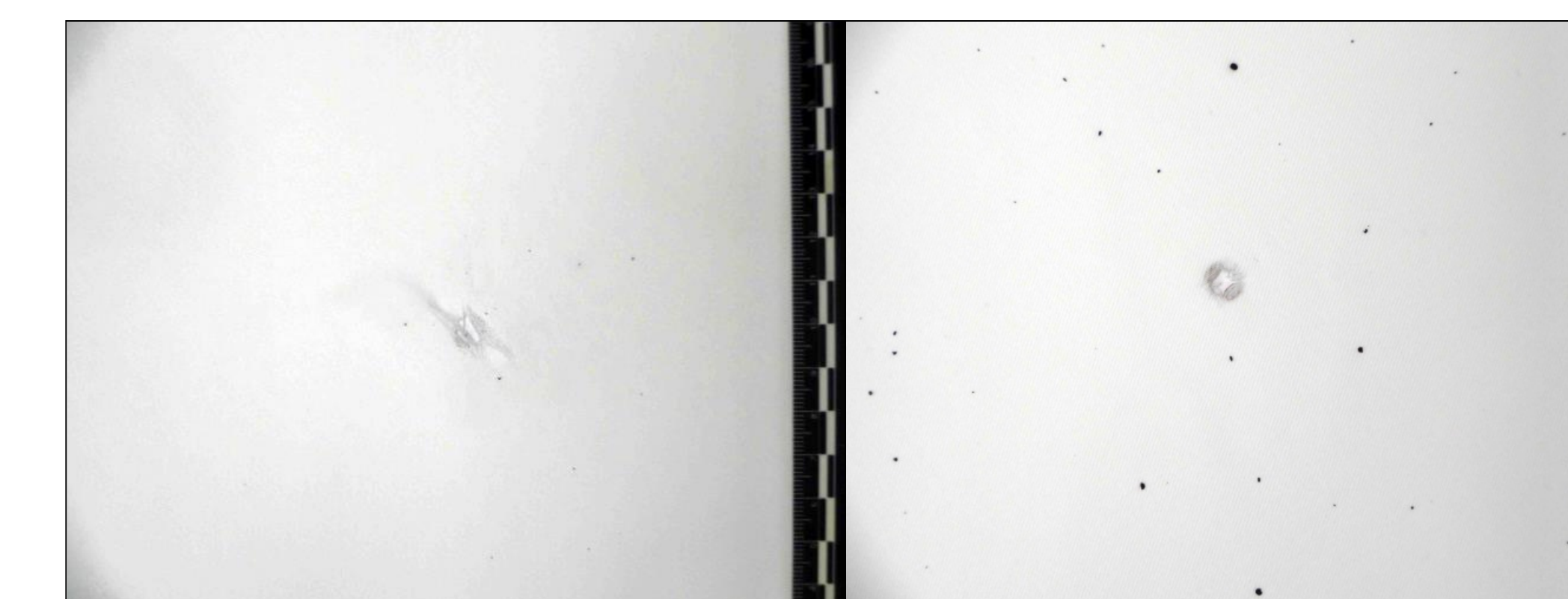
Figure 1 Side by side GSR pattern comparison of 3.5 grain Clays loaded cartridge at 12" (left) and a 12.0 grain Blue Dot loaded cartridge at 30" (right).
