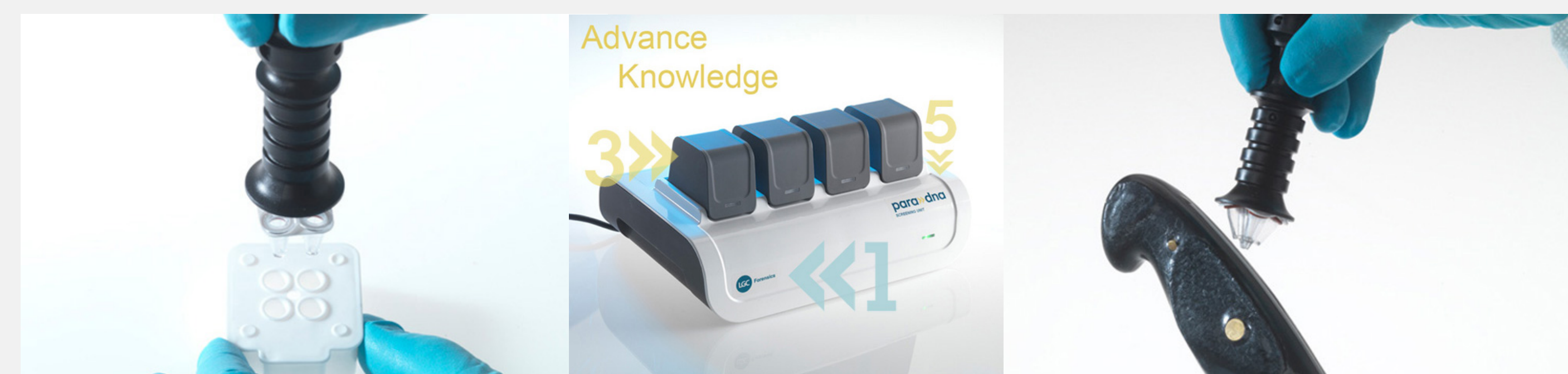
Figure 1: ParaDNA® Screening Kit Cartridge, Screening Instrument, and Sample Collector
