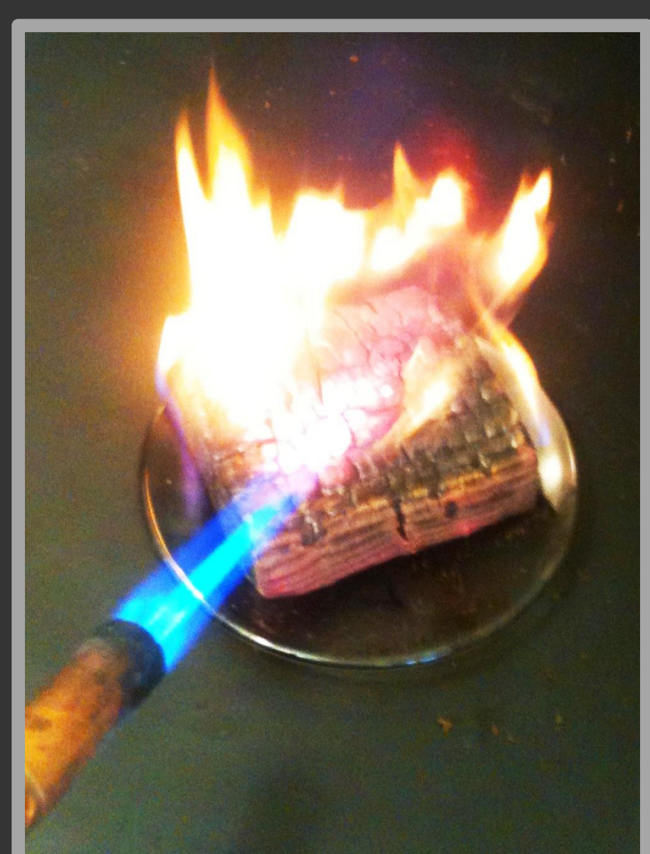
Figure 1. Propane torch charring of wooden sample.
