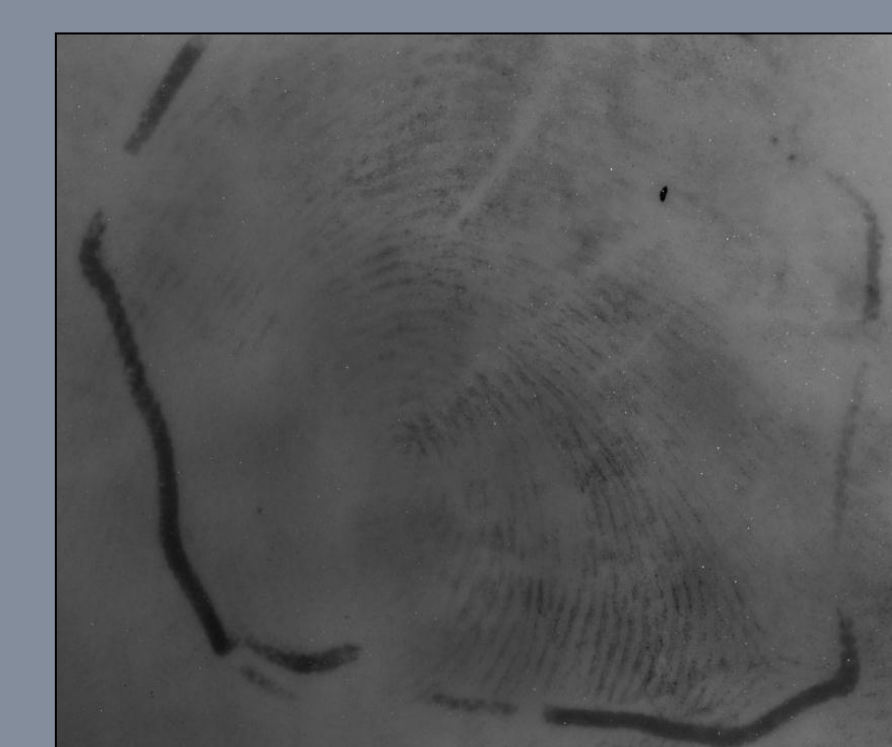
Figure 7. Print with a Score of 3, Developed with Cyanoacrylate in Week 2
