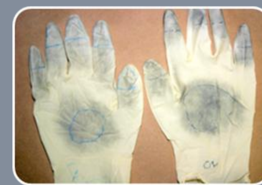
Fig 2. Gloves Processed with CA and Powder
