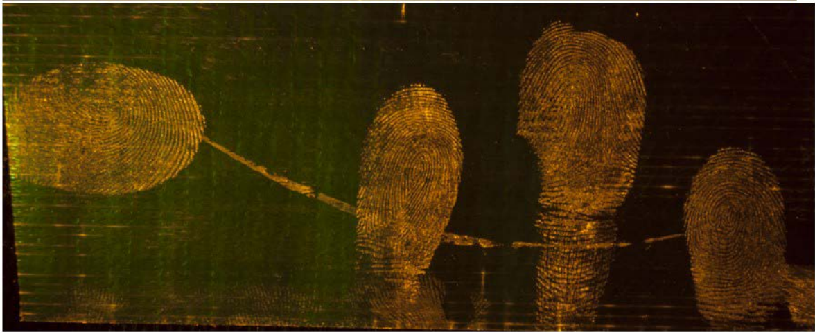
Figure 8- Duct tape processed in a solution of 0.05 g/L rhodamine 6G and 10% Tween 20.
