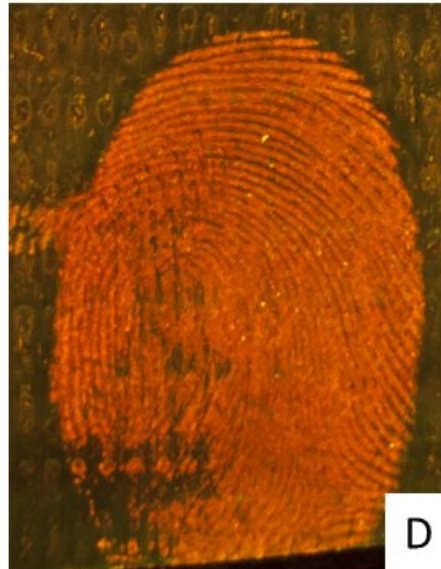
Figure 7- Duct tapes processed with A) TapeGlo, B) Wetwop, C) black powder, and D) rhodamine 6G.
